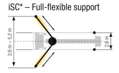
Dimensions can differ depending on configuration. Support width based on center of support leg. Diameter of swivel plate 270 mm.
