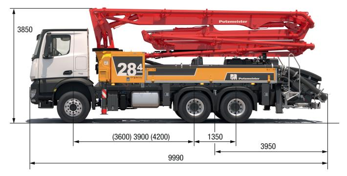
Note: Standard version. Dimensions and weights depend on truck, pump model and equipment. Dimensions in mm. Example based on Mercedes Benz Arocs 2636 with a 15 i LS core pump. For illustration only.
